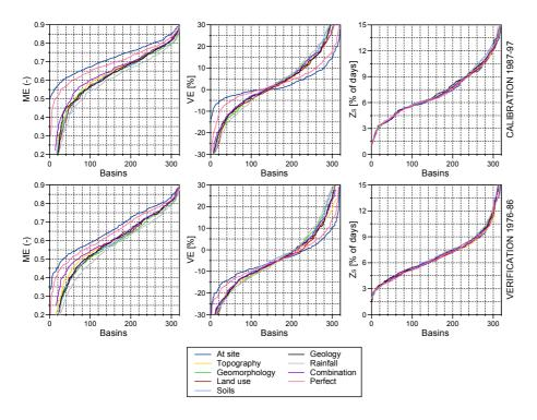
**Fig. 7.** Performance of the similarity index group of regionalisation methods: Cumulative distribution functions (*CDF*) of the model efficiencies of daily runoff (*ME*, left), volume errors of runoff (*VE*, centre) and percentage of days with poor snow cover simulations ( $Z_S$ , right). 320 basins, calibration (top) and verification (bottom) periods.
