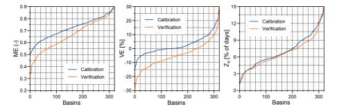
**Fig. 2.** At-site calibration and verification performances: Cumulative distribution functions (*CDF*) of the model efficiencies of daily runoff (*ME*, left), volume errors of runoff (*VE*, centre) and percentage of days with poor snow cover simulations ( $Z_S$ , right). 320 basins, calibration (1987–1997) and verification (1976–1986) periods.
