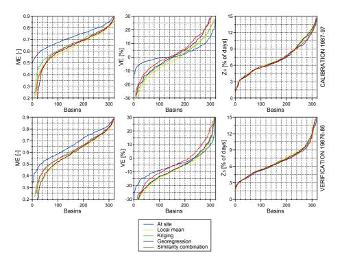
**Fig. 8.** Summary of the performance of the best regionalisation methods of each group: Cumulative distribution functions (*CDF*) of the model efficiencies of daily runoff (*ME*, left), volume errors of runoff (*VE*, centre) and percentage of days with poor snow cover simulations ( $Z_S$ , right). 320 basins, calibration (top) and verification (bottom) periods.
