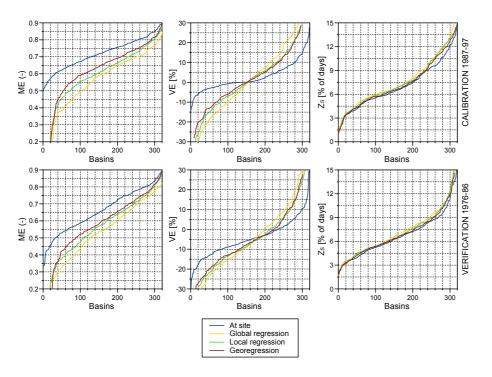
**Fig. 6.** Performance of the multiple regression group of regionalisation methods: Cumulative distribution functions (*CDF*) of the model efficiencies of daily runoff (*ME*, left), volume errors of runoff (*VE*, centre) and percentage of days with poor snow cover simulations ( $Z_S$ , right). 320 basins, calibration (top) and verification (bottom) periods.
