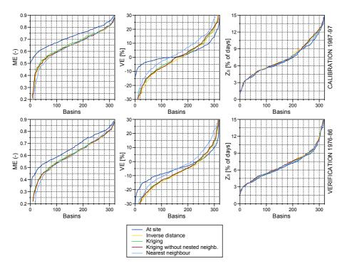
**Fig. 5.** Performance of the spatial proximity group of regionalisation methods: Cumulative distribution functions (*CDF*) of the model efficiencies of daily runoff (*ME*, left), volume errors of runoff (*VE*, centre) and percentage of days with poor snow cover simulations ( $Z_S$ , right). 320 basins, calibration (top) and verification (bottom) periods.
