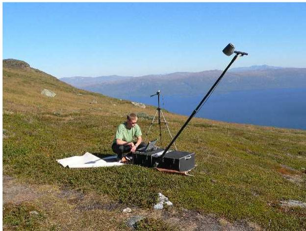
**Fig. 2.** Figifigo measuring BRF in Abisko, Sweden.
