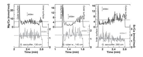
**Fig. 10.** Time-resolved LA-ICP MS Mg/Ca and Sr/Ca ratios of cleaned foraminiferal samples with diagenetic overgrowths of site SO164–19–2: Sample 130 cm (~260 kyrs), sample 145 cm (~288 kyrs), sample 260 cm (~473 kyrs). For detailed description, see Fig. 9.
