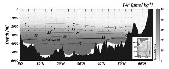
**Fig. 7.** Model results from the MIT ocean model, output as annual mean. – Meridional section of excess dissolved  $CaCO_3$ , TA\*, and the saturation horizon of calcite in the North Atlantic along A16. TA\* is defined as alkalinity from dissolution of  $CaCO_3$  below the surface layer and is normalized to the moles of calcium carbonate that have been dissolved.
