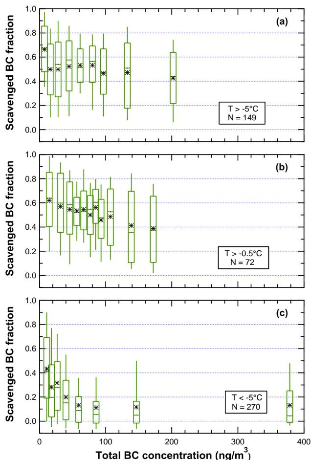
**Fig. 4.** Dependence of the scavenged BC fraction on the BC concentration measured downstream of the total inlet at  $T > -5^{\circ}\text{C}$  based on 224 h of in-cloud measurements (a), at  $T > -0.5^{\circ}\text{C}$  (b, 132 h) and at  $T < -5^{\circ}\text{C}$  (c, 360 h).
