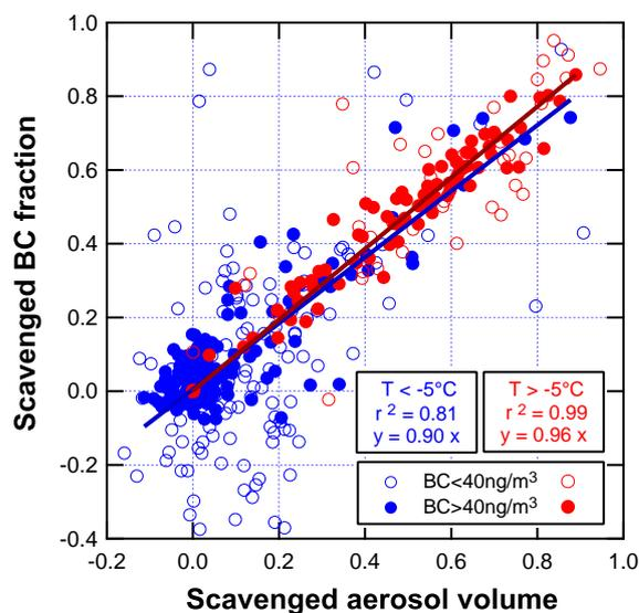
**Fig. 7.** Correlation between the scavenged BC fraction and the scavenged bulk volume fraction for  $T < -5^\circ\text{C}$  (blue dots) and  $T > -5^\circ\text{C}$  (red dots). Data with low concentrations (open circles; BC concentrations  $< 40 \mu\text{g}/\text{m}^3$ ) were excluded from the correlation analysis.
