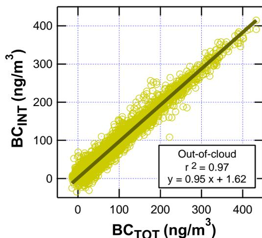
**Fig. 1.** Comparison of the BC concentrations (determined by two MAAPs) from the total and interstitial inlet during clear sky conditions ( $CWC < 0.01 \text{ g/m}^3$ ) for 1800 h of measurements. Symbols represent 10-min averages.
