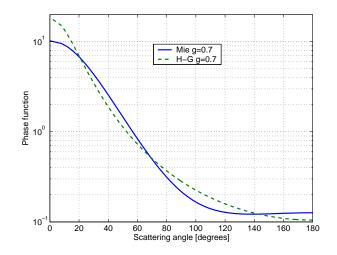
**Fig. 2.** Mie and Henyey-Greenstein phase function with the same asymmetry factor (g=0.7).
