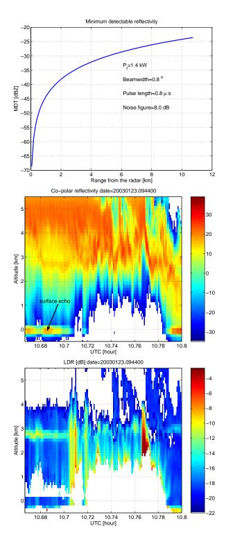
**Fig. 13.** Top panel: minimum detectable reflectivity for the ACR system (relevant specifications are also listed). Detail of the copolar reflectivity (center panel) and the LDR (bottom panel) as measured by the ACR during the Wakasa Bay Experiment on the 23 January 2003.
