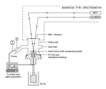
**Fig. 13.** Experimental set-up for FTIR spectroscopic measurements of stratospheric condensates in contact with the gas-phase.
