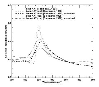
**Fig. 2.** The effect of reduced spectral resolution on refractive indices of  $\beta$ -NAT in the region of the  $\nu_2$ -band of NO $_3^-$ . Biermann (1998)'s data which have been obtained with a resolution of 1 cm $^{-1}$  have been smoothed to be comparable with the measurements by Toon et al. (1994).
