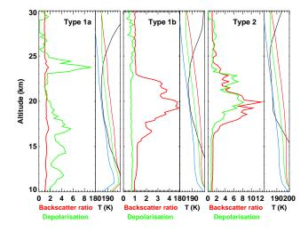
**Fig. 3.** Backscatter ratio and depolarization profiles of three Lidar measurements of different PSC Types which were selected for analysis of PSCs from matching MIPAS limb-scans (see Table 2). Corrected ECMWF temperature profiles are black (see text and Appendix B for details). Existence temperatures are colour-coded: blue for ice, green for STS, and red for NAT.
