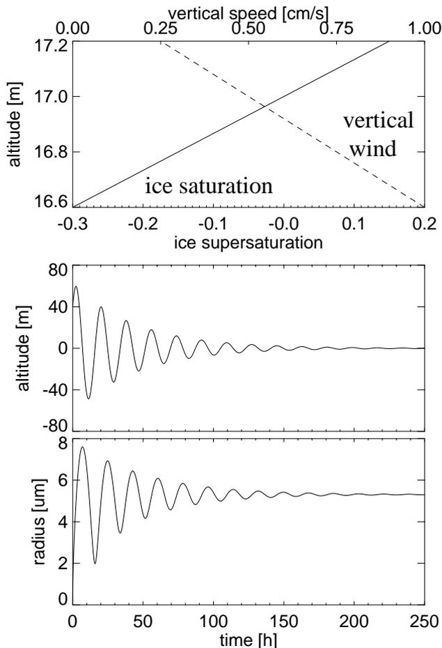
**Fig. 2.** One-particle simulation. Upper panel: prescribed ice saturation ratio and wind profile used for the calculation. Middle and lower panel: the altitude and size evolution of a small ice particle released 40 m above the equilibrium level.
