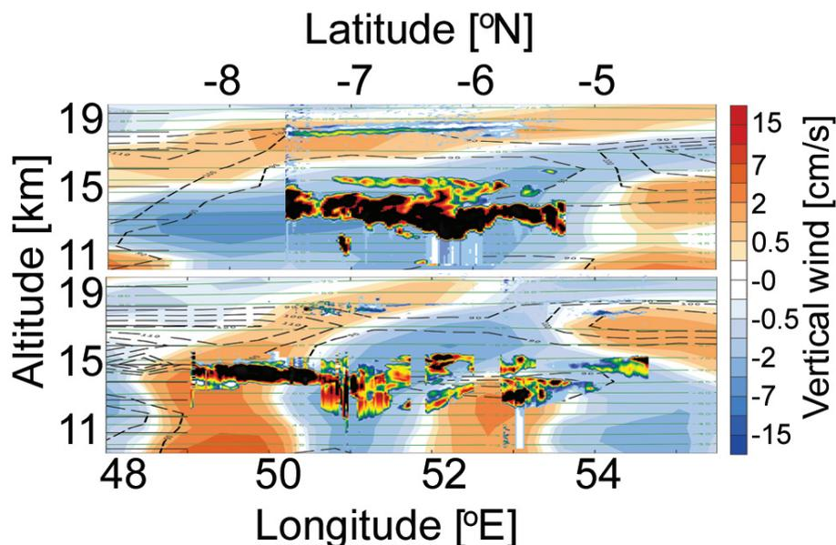
**Fig. 6.** Similar to Fig. 5, but for 24 February 1999. The top panel shows the North-South flight leg and the lower panel the East-West rebound flight leg on that day. The noise of the lidar signal at  $\sim 50.5^\circ$  E was due to icing of the windows of the lidar instrument. UTTCs are clearly visible around 18 km altitude, but only in regions with upwelling (reddish colours) and sufficient moisture (dashed lines corresponding to  $S_{\text{ice}} = 90\%$ ,  $100\%$  and  $110\%$ ).
