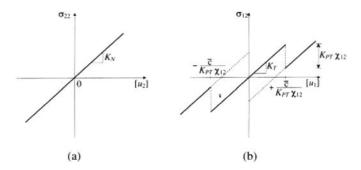
FIG. 4. Contact laws for c>0: (a) normal contact law for  $\chi_{22}=0$ ; (b) tangential contact law.
