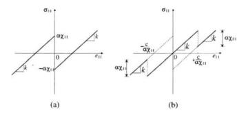
FIG. 2. Stress-strain diagrams obtained in an extension test on the adhesive: (a)  $c \le 0$ , (b) c > 0.
