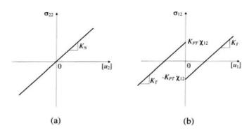
FIG. 3. Contact laws for  $c \le 0$ : (a) normal contact law for  $\chi_{22} = 0$ ; (b) tangential contact law.
