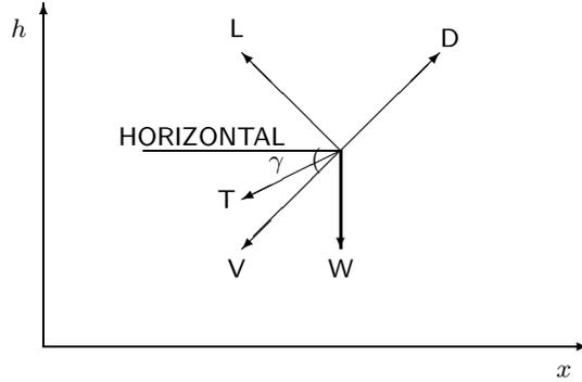
FIGURE 1. Aircraft forces during phase of descent
