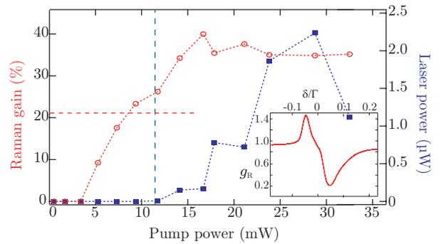
FIG. 3: Laser power (squares) and Raman gain (open circles) versus pump power, with  $b_0 = 10$  and  $\Delta = -7\Gamma$ . Lasing threshold (vertical dashed line) is expected to appear with a gain of about 21% (horizontal dashed line), in good agreement with the experimental data. Inset: Typical weak-probe transmission spectrum.
