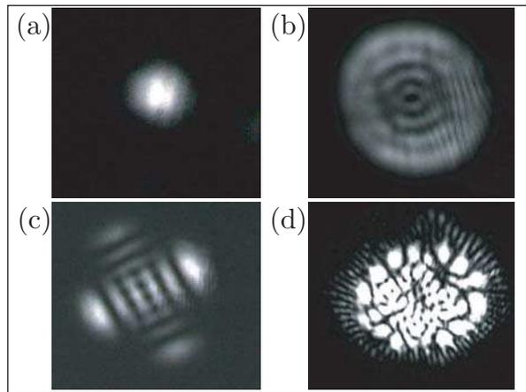
FIG. 1: Transverse modes of cold-atom lasers. (a) Gaussian  $TEM_{00}$  mode, obtained by inserting a small diaphragm in the cavity. Typical modes of (b) the Mollow laser, (c) the Raman laser, and (d) the four-wave mixing laser.
