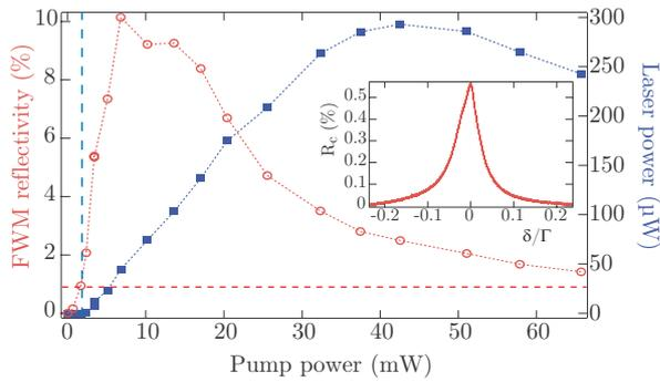
FIG. 4: Laser power (squares) and phase-conjugate reflectivity due to four-wave mixing (open circles) versus pump power, with  $b_0 = 10$  and  $\Delta = -8\Gamma$ . Lasing threshold (vertical dashed line) is expected for a reflectivity around 1% (horizontal dashed line), in good agreement with the experimental data. Inset: Example of a weak-probe reflectivity spectrum.
