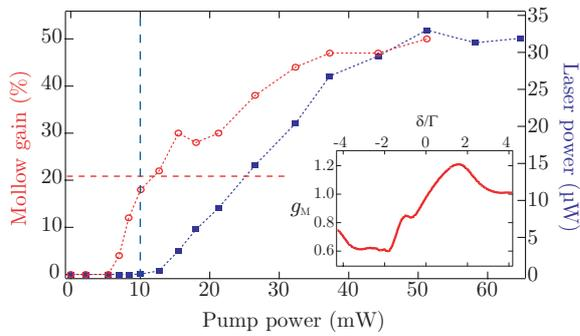
FIG. 2: Laser power (squares) and Mollow gain (open circles) versus pump power, with  $b_0 = 11$  and  $\Delta = +\Gamma$ . Lasing threshold (vertical dashed line) is expected to appear with a gain of about 21% (horizontal dashed line), in good agreement with the experimental data. Inset: Typical weak-probe transmission spectrum.
