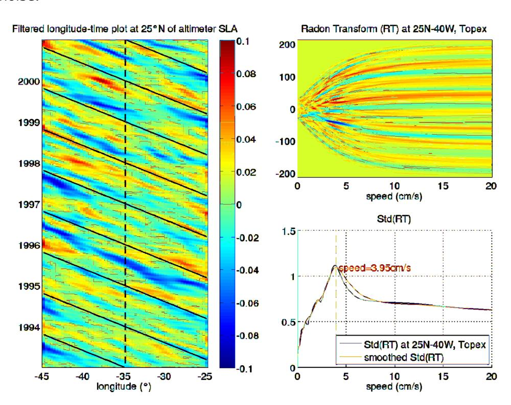
This method allows to quantify the zonal phase speeds C(x,y,z) of the dominant signal at each location (x,y,z) (black dots in the figure below). An EOF analysis and a comparison with theoretical phase speeds (Killworth et al. 2003 white dots) show that the dominant signal corresponds to the first baroclinic mode of Rossby waves. Phase speeds of the second and higher modes are detected too (black circles).
