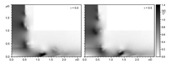
FIG. 24. Time sequence of the phase-averaged velocity fields for two-frequency excitation ( $St_e = 1.60$  and 0.80).
