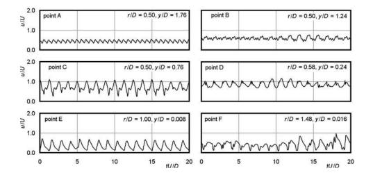
FIG. 21. Velocity signals measured at the different locations inside the excited impinging jet ( $St_e=1.6$ ). See Fig. 20 for the measuring point's localization.
