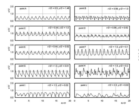
FIG. 16. Velocity signals measured at different locations inside the excited impinging jet ( $St_e$ =0.74). See Fig. 15 for the point's localization.
