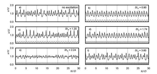
FIG. 5. Velocity signals measured in the near-wall region (r/D=1, y/D=0.04) at the different jet excitation frequencies. The sinusoidal excitation signals are shown at the bottom of each graph (excitation amplitude and phase are not to scale).
