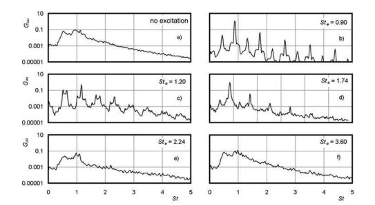
FIG. 6. Power spectra of near-wall velocity fluctuations calculated for data presented in Fig. 5.
