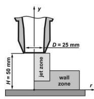
FIG. 4. Coordinate system for the impinging jet and measuring zones.
