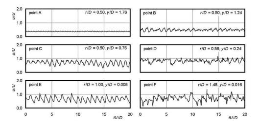
FIG. 23. Velocity signals measured at different locations inside the excited impinging jet ( $St_e$ =2.14). See Fig. 22 for the point's localization.
