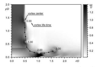
FIG. 13. Vortex trajectory inside the excited impinging jet ( $St_e=0.74$ ) determined from a sequence of phase-averaged velocity fields. Vortex lifetime is expressed as a number of excitation periods elapsed from the vortex formation.
