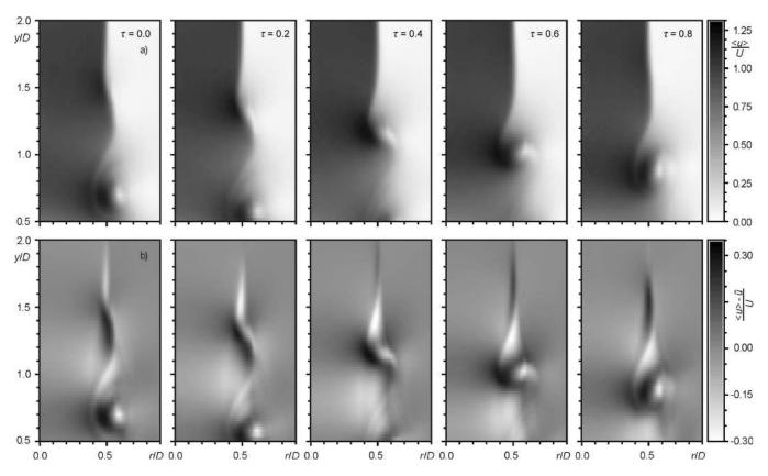
FIG. 11. Evolution of the phase-averaged velocity field in the excited jet zone (St<sub>e</sub>=0.74): (a) phase-averaged velocity and (b) difference between phase-averaged and time-averaged velocity.  $\tau = tf_e$  is a particular phase of the excitation period.
