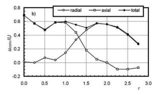
FIG. 14. Vortex convection velocity as a function of the vortex lifetime in the excited impinging jet ( $St_e=0.74$ ). The axial velocity component has an inverted sign with positive values for the movement toward the wall.
