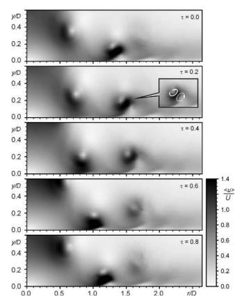
FIG. 12. Evolution of the phase-averaged velocity field in the wall jet region of the excited jet ( $St_e=0.74$ ).
