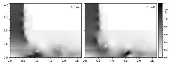
FIG. 25. Time sequence of the phase-averaged velocity fields of a jet excited at two frequencies ( $St_e = 1.60$  and 0.53).
