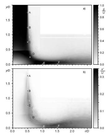
FIG. 22. Time-averaged velocity fields for the excited impinging jet (St<sub>e</sub> = 2.14): (a) time-averaged velocity and (b) velocity rms.
