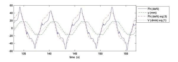
**Figure 3 :** In-line force obtained from the Morison equation (Fh eq.3) against flow velocity at the bottom (V eq.1) and measured horizontal force (Fh) against horizontal displacement (y) for load controlled test L8. Forces are in daN, with 1 daN = 10 N.
