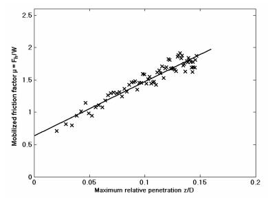
Figure 22: Evolution of the mobilized friction factor  $\mu$  with pipe penetration during Test D8.
