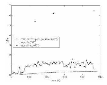
**Figure 13:** Excess pore pressure at  $60^{\circ}$  under the pipe compared to effective vertical stress and passive pressure stress at the same depth during penetration of the pipe. Load controlled test L8. Load amplitude 600 N, period T = 6 s.
