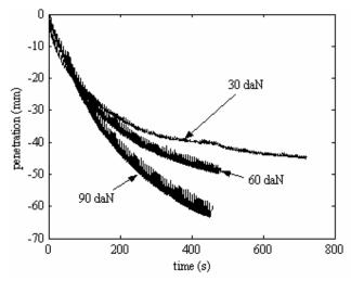
**Figure 8:** Influence of the load-amplitude on the penetration of the pipe, for a period T=6 s. Dense sand. 1daN = 10 N.
