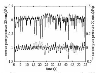
**Figure 19:** Recording of the pore pressure transducers placed within the soil. Controlled displacement test D3, performed with the electro-mechanical actuator set. Period T = 1.5 s
