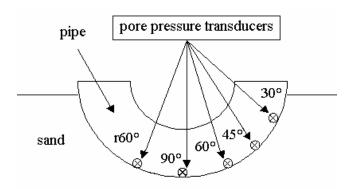
Figure 4: Distribution of the pore pressure sensors along the pipe-soil interface
