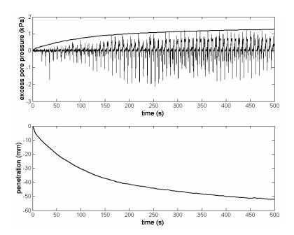
**Figure 14:** Load controlled test. Amplitude 600 N, period T = 8 s. Dense sand.
