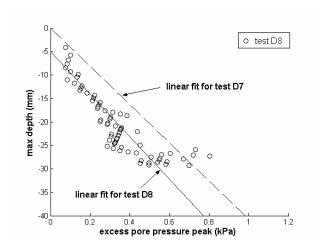
**Figure 15:** Development of excess pore pressure with pipe penetration. Loose sand. Tests D7 and D8.
