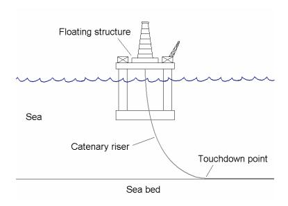
**Figure 1:** Wave-induced cyclic loading of a catenary riser on the seabed.
