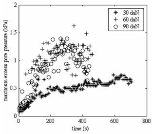
**Figure 9:** Influence of the load amplitude on the maximum excess pore pressure at  $60^{\circ}$  during each cycle. Period 6 s. Dense sand. 1 daN = 10 N.
