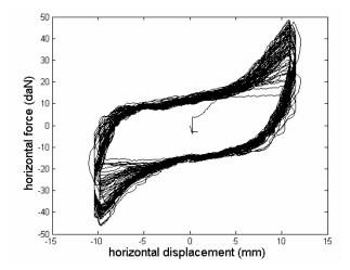
**Figure 12:** Cyclic load-displacement curves for Test D8 with amplitude  $\pm 10.5$ mm, T=4.55s.
