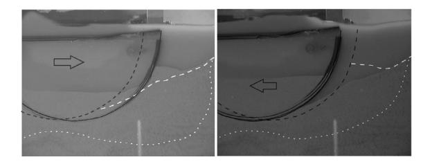
**Figure 20:** Video frames 1 s apart at the maximum excursion of the pipe (controlled force test L4, maximum applied horizontal force: 500 N, T=2s). The pipe position and soil/water interface at the preceding half-period are plotted with dashed line (black and white respectively). The dotted line bounds the area where grain motion was observed during the preceding half-period.
