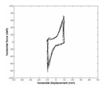
**Figure 11:** Cyclic load-displacement curves for displacement-controlled test D2 with an amplitude of 10 mm and a period of 2 s.
