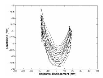
Figure 10b: Cyclic penetration-horizontal displacement curves of the pipe. Test L8.
