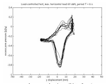
**Figure 16:** Cyclic pore pressure changes at the pipe-soil interface (sensor at 60°), test L8.
