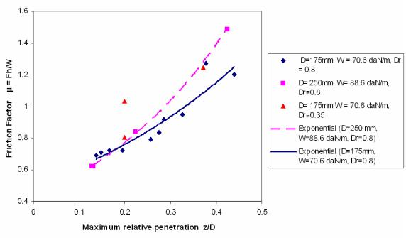
**Figure 21:** Equivalent friction factors obtained by Branque et al (2002)
