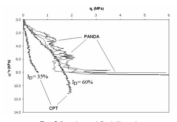
**Figure 5 :** Penetration curves in Fontainebleau sand.
