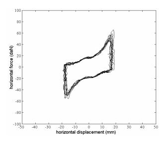
**Figure 10a.** Cyclic load- horizontal displacement curves for Test L8. Load amplitude 600 N. Period 6 s.
