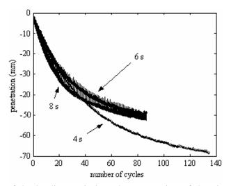
Figure 6: Influence of the loading period on the penetration of the pipe. Maximum applied
