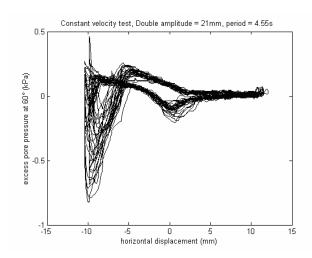
**Figure 17:** Cyclic pore pressure changes at the pipe-soil interface (sensor at 60° left). Test D8 (loose sand).
