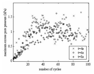
Figure 7: Influence of the loading period on the excess pore pressure at 60° under the pipe.
