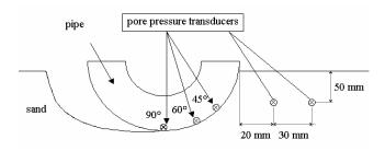
Figure 18: Location of the pore pressure sensors along the pipe and in the soil
