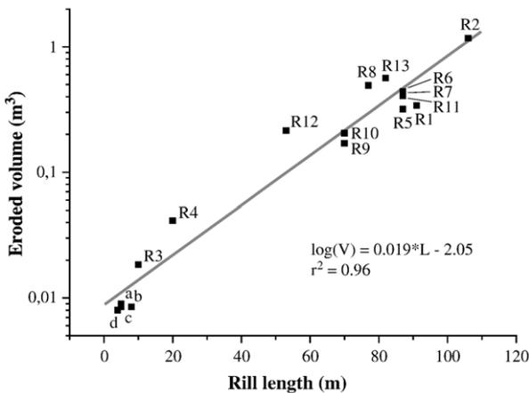
Fig. 7. Relationship between eroded volume and rill length.
