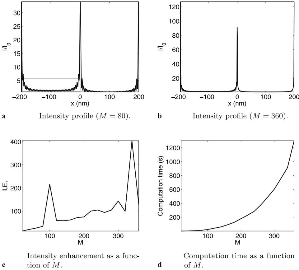
**FIGURE 3** The intensity enhancement computed from CWM for a grating with aspect ratio 0.5, height 20 nm, and period 400 nm. The angle of incidence of the incoming light is 0. The intensity enhancement is computed 2 nm above the grating tracks
