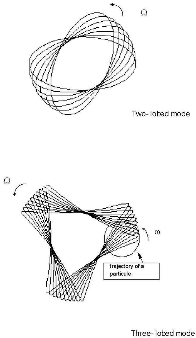
Fig. 1. In the case of two-lobed mode or three-lobed mode, the drops are turning around their centre of symmetry. The trajectory of a particle is a circle represented in the case of a three-lobed mode.
