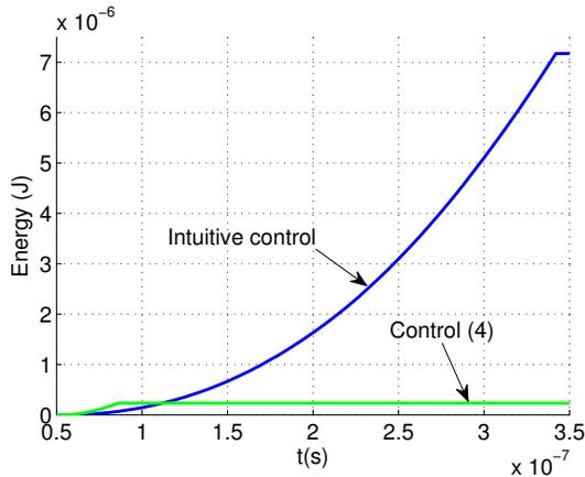
Fig. 7: Energy dissipated during the rising transient period.
