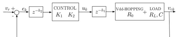
Fig. 2: Block diagram of the circuit control system.
