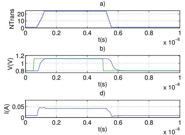
Fig. 3:  $R_0 = 31.41\Omega \rightarrow R_0 = 37.7\Omega$ ,  $K_1 = -0.47$ ,  $K_2 = 0.68$ . Evolution of the: a) number of transistors switched on, b)  $v_r$  (dashed) and  $v_c$  (solid), c) current  $I_l$ .
