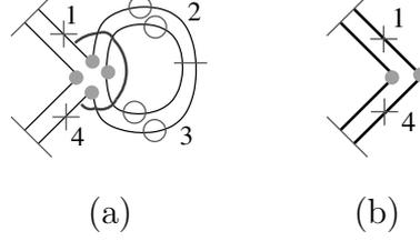
Fig. 5. 1-removal in 2D of a loop. (a) Initial 2-G-map. (b) Result. For instance,  $1\alpha'_1 = 1(\alpha_1\alpha_2)(\alpha_1\alpha_2)\alpha_1 = 4 \in B^S$  (since  $1(\alpha_1\alpha_2)\alpha_1 \notin B^S$ , this dart belongs either to  $C$  and to  $C\alpha_1$ ).
