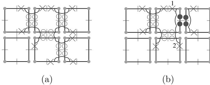
Fig. 8. (a) Simultaneous 1-removals in 2D. (b) Simultaneous 1-removals (dart marked with circles) and 1-contractions (dart marked with black disks) in 2D. For instance,  $1\alpha'_1 = 1(\alpha_1\alpha_0)(\alpha_1\alpha_2)\alpha_1 = 2$  since the edge incident to  $1\alpha_1$  is contracted and the edge incident to  $1(\alpha_1\alpha_0)\alpha_1$  is removed.
