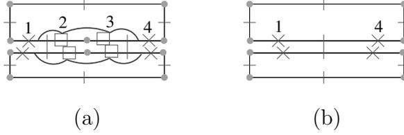
Fig. 3. 0-removal in 2D. (a) Initial 2-G-map. (b) Result.  $C = \langle \alpha_1, \alpha_2 \rangle$  (2) (darts marked with empty squares),  $C\alpha_0 = B^S$  (darts marked with crosses). For instance,  $1\alpha'_0 = 1(\alpha_0\alpha_1)\alpha_0 = 4 \in B^S$
