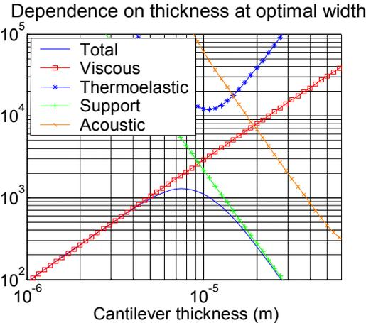
**Figure 3:** Quality factors (log scale) at the optimal width (37 μm) for a 100 μm long microcantilever as a function of the thickness (log scale)
