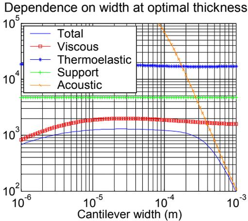
**Figure 4:** Quality factors (log scale) at the optimal thickness (7.7 μm) for a 100 μm long microcantilever as a function of the width (log scale)
