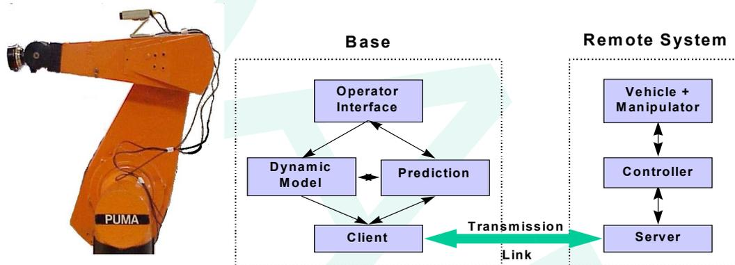
Figure 3: PUMA arm and enhanced teleoperation structure
