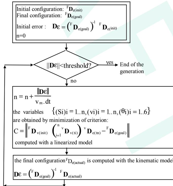
Figure 7: Implemented algorithm («o» denotes the composition of two transformations)
