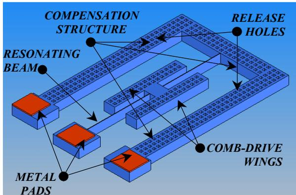
Fig. 3.1: A 3D view of the resonator
