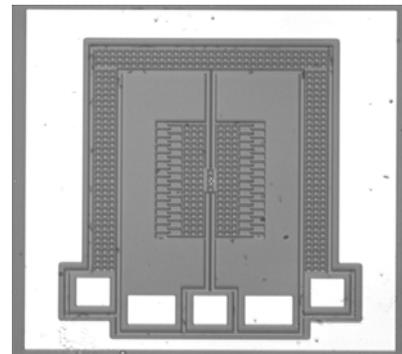
Fig. 5.1 The top view of the fabricated structure (resonator)
