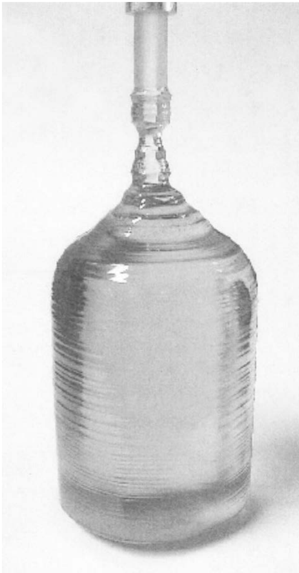
Fig. 1. Example of an as-grown Nd:YCOB crystal. Some growth striation is still visible inside the crystal.
