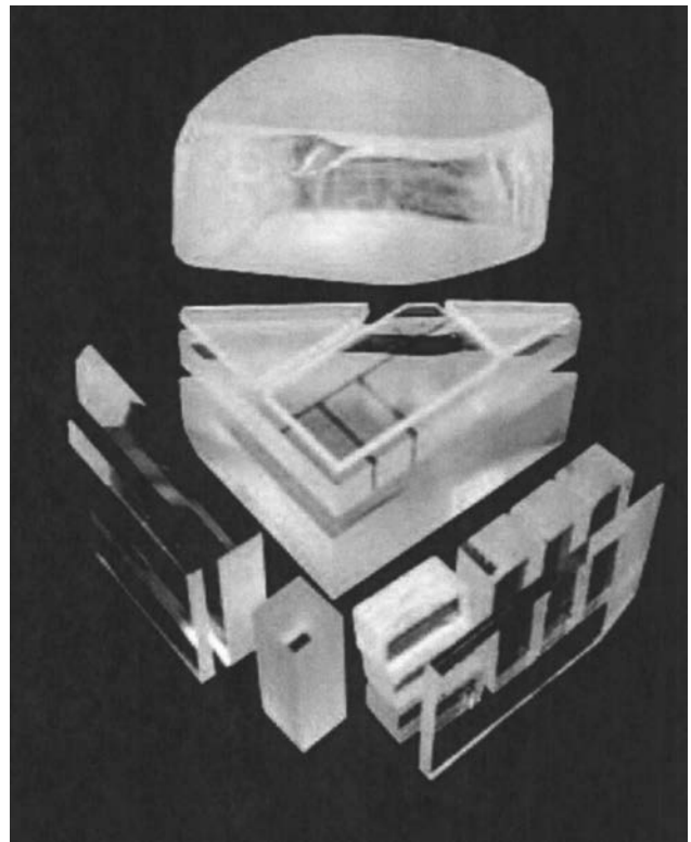
Fig. 2. Block and the oriented pieces that were cut and polished along the crystallographic axis in a YCOB slab.
