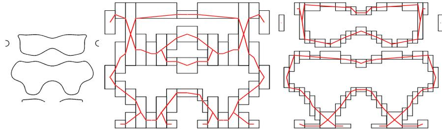
**Fig. 7.** The function  $x^2 + y^2 + \cos(2\pi x) + \sin(2\pi y) + \sin(2\pi x^2) \cos(2\pi y^2) = 1$  on  $[-1.1; 1.1] \times [-1.1; 1.1]$  (*left*) discretized by an algorithm described in [24] with two different resolutions, then recoded and polygonalized (*center and right*)
