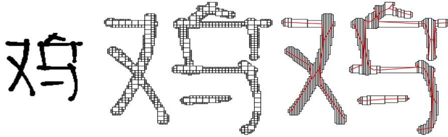
**Fig. 6.** An image of a chinese character (*left*), compressed by a quadtree-based approach (*center*). We show the final  $k$ -arcs recoding and the polygonalization (*right*)
