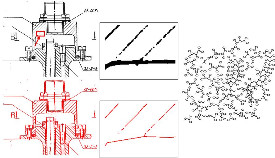
**Fig. 8.** An image of technical drawing of size 1765 x 1437 pixels we submit to our system, and a zoomed part of it, indicated by the arrow (*up*). The polygonalization we obtain and the associated zoom are presented (*bottom*). The complete Reeb graph (about 300 nodes) is also illustrated in a circular format (*right*)
