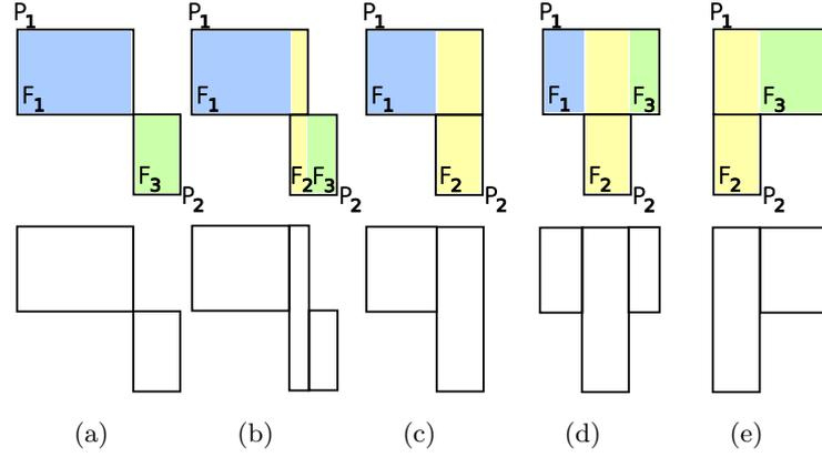
**Fig. 3.** Description of rectangles  $F_1$ ,  $F_2$  and  $F_3$  in the update procedure (top), and the associated cells as result (bottom). When  $P_1^R < P_2^R$  (a and b),  $P_1 - F_2 = F_1$  and  $P_2 - F_2 = F_3$ , else  $P_1 - F_2 = \{F_1, F_3\}$  (d and e). If  $P_1^R = P_2^R$ ,  $F_2 = \emptyset$ , when  $P_1^R = P_2^R$ ,  $F_3 = \emptyset$  and finally  $F_1 = \emptyset$  in the case  $P_1^L = P_2^L$
