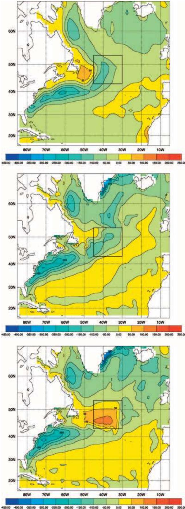
◀ **Fig. 11** Net surface heat flux ( $\text{Wm}^{-2}$ , mean 1988–1997). *Top* NCEP/NCAR reanalysis data; *middle* experiment NCEP1; *bottom* experiment NCEP2. Figures from our experiments include the effect of the SST retroaction term. The *box* indicates the region discussed at the end of Section 4.1
