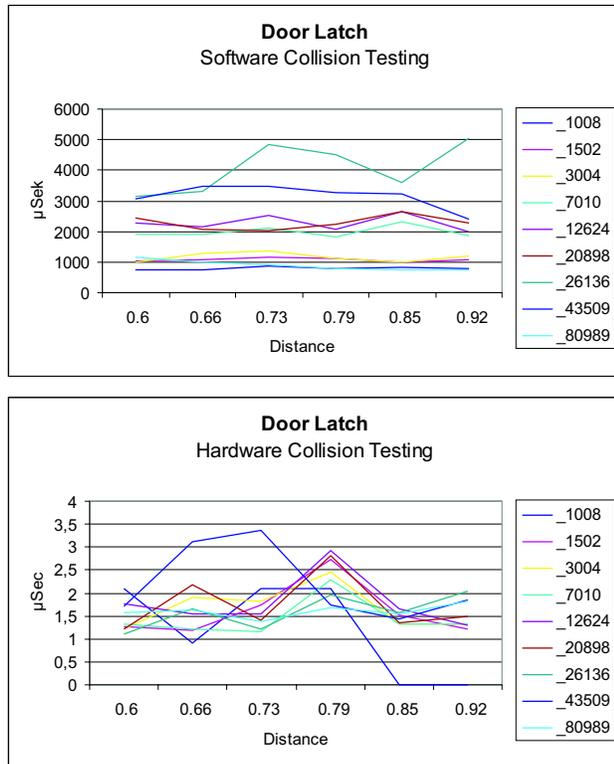
**Figure 8. Comparison of software with hardware implementation at various distances and polygon complexities. Our collision detection architecture is up to 1000 times faster in determining all intersecting triangles of two objects than the software implementation running on a 1GHz Pentium 3.**
