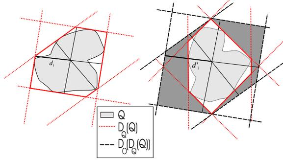
**Figure 1. Our DOP overlap test gains its speed by transforming DOP Q into O's reference frame  $F(O)$ . The tightness loss is shown in dark grey. Obviously, each  $d'$  is determined by exactly three original  $d$ 's.**
