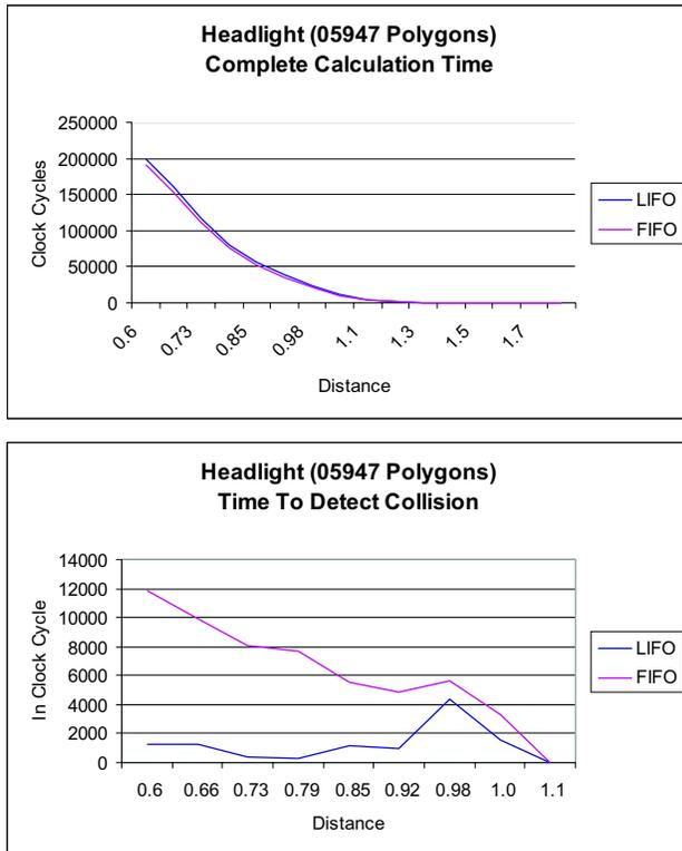
**Figure 6. Top: Comparing LIFO and FIFO controlled intersection testing shows that finding all intersecting primitives takes equally long. Bottom: Our comparison shows that LIFO control is far superior to FIFO control when finding the first intersecting primitive.**
