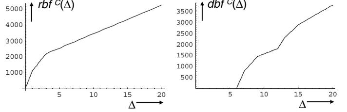
Figure 5: Composite resource and demand bound functions corresponding to the task graph  $g_1$  in Figure 2 and the arrival function shown at the right hand side of Figure 3.
