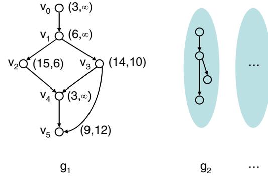
Figure 2: Only one sample task graph  $g_1 \in G$  is shown in detail. Each node  $v_i$  of  $g_1$  is associated with a tuple  $(c(v_i), d(v_i))$ , where  $c(v_i)$  is the node’s worst case resource demand and  $d(v_i)$  is its relative deadline.
