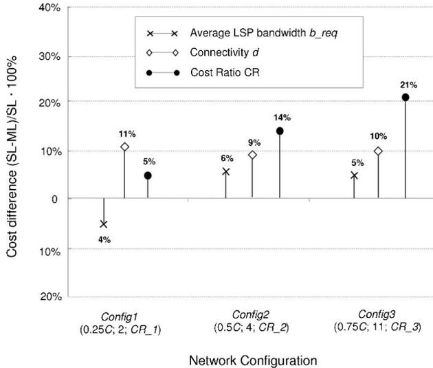
Fig. 10. Relative cost difference  $\left(\frac{SL-ML}{ML} \cdot 100\%\right)$  between SL and Interlayer BRS (ML) survivability for different values of input parameters: LSP traffic granularity, network connectivity and cost.
