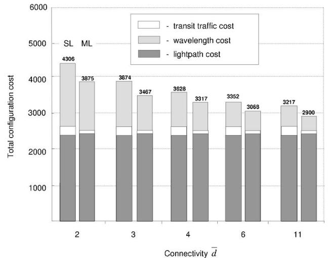
Fig. 9. SL vs. Interlayer BRS (ML) survivability for different physical topologies. Traffic matrix consisting of 126 LSPs; average LSP bandwidth=0,5C; 12-node physical network; cost ratio CR<sub>1</sub>.
