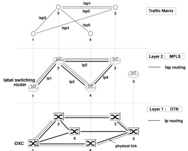
Fig. 1. Architecture of the MPLS over OTN.
