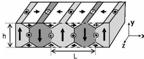
Fig. 2. Schematic representation of the stripe structure in a thin film.
