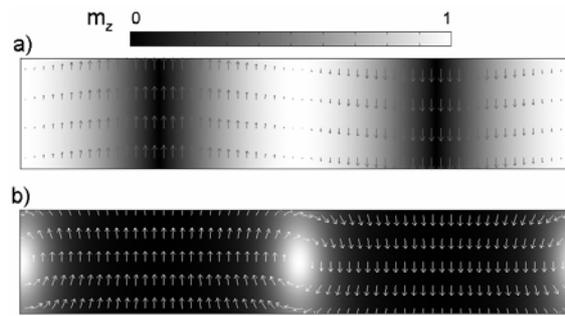
Fig. 3.a) The initial magnetic configuration. b) The equilibrium magnetization distribution calculated by FEM. For both a) and b) the  $m_x$  and  $m_y$  magnetization components are represented by arrows and the  $m_z$  component by a grey scale. Material parameters:  $A_{ex}=2 \cdot 10^{-11}$  J/m,  $\mu_0 M_s=1$  T and  $K_1=10^5$  J/m<sup>3</sup>.
