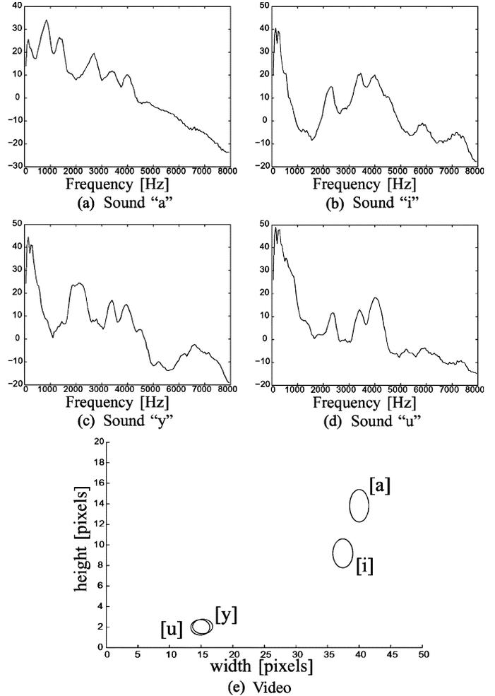
Fig. 7. Illustration of the corpus. Figs. (a), (b), (c), (d) present the audio kernels  $[(\sigma_i^A(f_1))^2, \dots, (\sigma_i^A(f_L))^2]^T$  (in decibels) interpreted as the psd of four French vowels [a], [i], [y], [u], respectively. (e) Corresponding video kernels.
