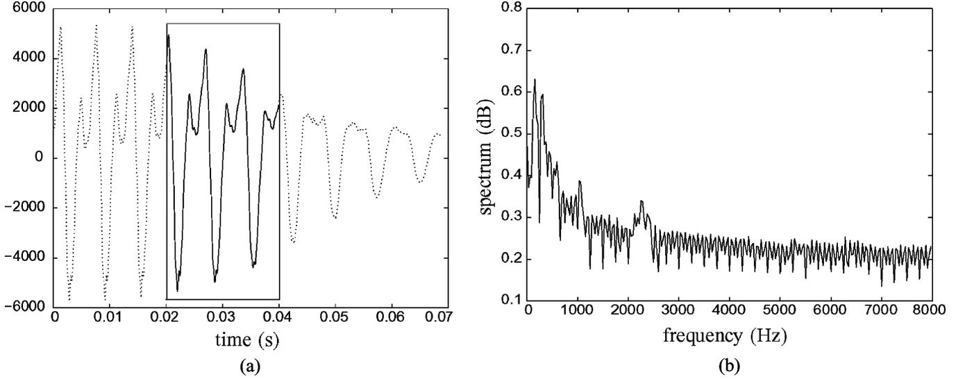
Fig. 4. Audio parameters. (a) Speech signal and the frame. (b) Spectrum of the frame.
