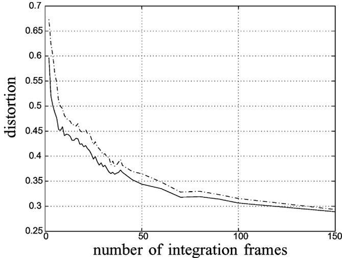
Fig. 8. Distortion (39) versus number of integration frames. Solid line: AV estimation (36) and dashed-dot line: audio estimation (31).
