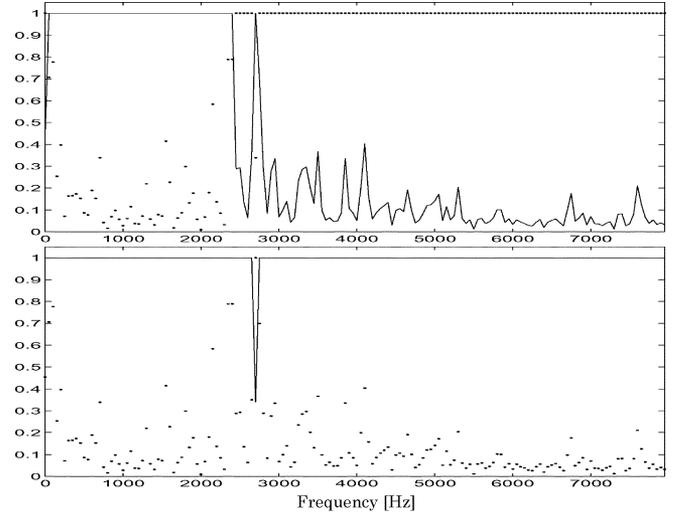
Fig. 12. Performance index  $r(f)$  [Eq. (40)] (dots) and its inverse (solid line) truncated at 1, before (upper panel) and after (lower panel) our ambiguities cancellation versus the frequency.
