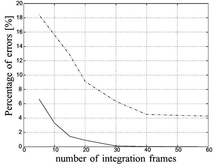
Fig. 9. Percentage of errors versus number of integration frames. Solid line: permutation of 250-Hz bandwidth blocks, dashed-dot line: permutation of 100-Hz bandwidth blocks.
