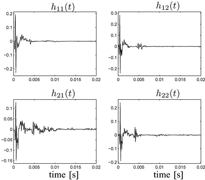
Fig. 11. Mixing filters: impulse response of the four mixing filters.
