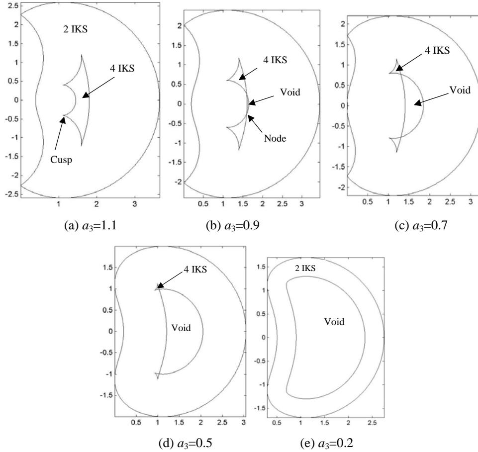
**Fig. 3 : Continuous deformation of the internal boundary as  $a_3$  is decreased ( $a_2=1.5, d_2=0.5$ ). From 1.1 to 0.5, the manipulator is quaternary (a-c). From 0.5 to 0.2, two cusps and one node merge into one point with four equal IKS and then disappear : the manipulator turns binary (d-e).**
