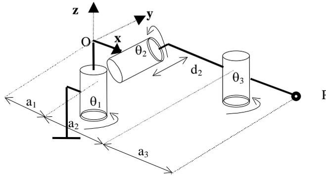
Fig. 1 : Orthogonal manipulator in its zero configuration
