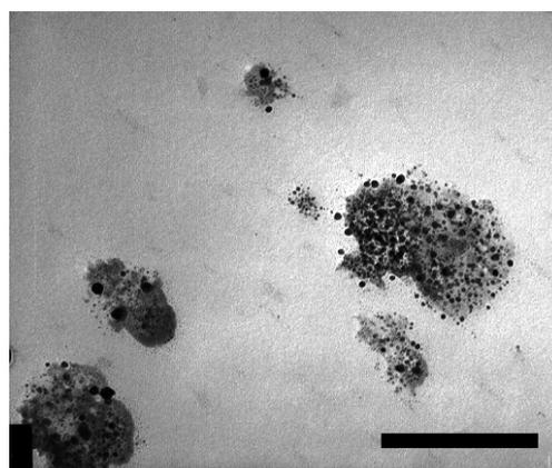
**Figure 2:** TEM picture of hybrid copolymer micelles loaded with magnetic nanoparticles obtained by combining PB<sub>48</sub>-b-PGA<sub>114</sub> and 1 mass equiv. of surfacted ferrofluid S2-CH<sub>2</sub>Cl<sub>2</sub>. The scale bar measures 400 nm.
