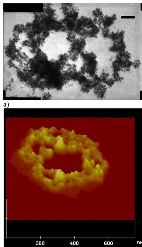
**Figure 4:** a) TEM picture of a magnetic membrane made of  $PB_{48}\text{-b-PGA}_{56}$  and 1 equiv. of  $S2\text{-CH}_2\text{Cl}_2$ . The scale bar measures 333 nm. b) 3-d view built from an AFM picture of the same sample (see Supplemental Information II) showing a flat copolymer membrane stuffed with magnetic iron oxide nanoparticles. Strong spreading on mica opens holes in the central part, whereas some pure copolymer bilayer is visible at the periphery.
