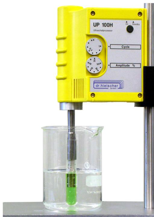
**Picture 1 – 100W Setup for Feasibility Testing**
