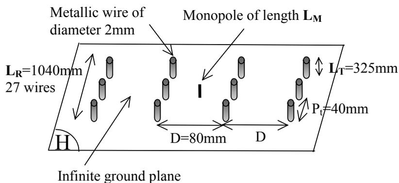
Figure 6 – Monopole inside the finite EBG structure
