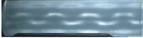
FIGURE 7. Pictures of the observed modes of elliptical instability depending on the global rotation \tilde{\Omega}^G for a given cylinder of radius \tilde{R} = 2.75 \text{ cm} and height \tilde{H} = 21.4 \text{ cm} with an eccentricity \varepsilon = 0.085 rotating at \tilde{\Omega}^F = 1.001 \pm 0.005 \text{ Hz} ( Re = 4.76 \times 10^3 ). In these pictures, the rotation axis is horizontal.
