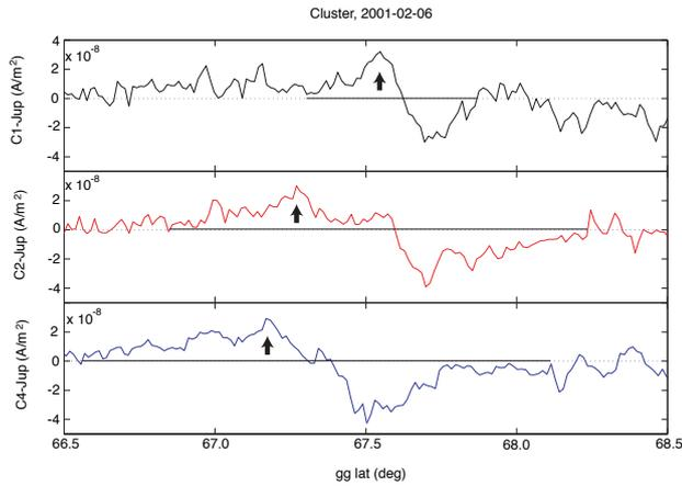
**Fig. 3.** FAC densities for C1, C2 and C4 as a function of geographic latitude, positive values mean upward current from the ionosphere. Arrows show the location of the maximum upward FAC and solid horizontal lines indicate the estimated widths of the current sheets. The times corresponding to arrows from top to bottom are: 23:24:10 UT, 23:25:25 UT and 23:27:20 UT.
