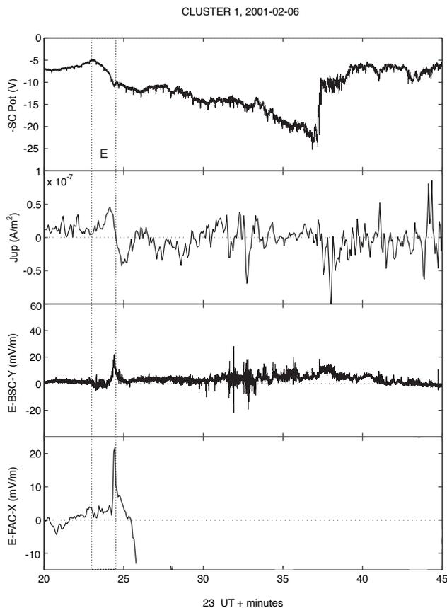
**Fig. 5.** Cluster 1 EFW and FGM measurements. Panels from top to bottom: Negative of the s/c potential, FAC density (positive away from the ionosphere), BSC-Y component of the high-resolution electric field (every 10th point shown) and FAC-X component of the DC electric field. The equatorward (poleward) arc are denoted by E (P).
