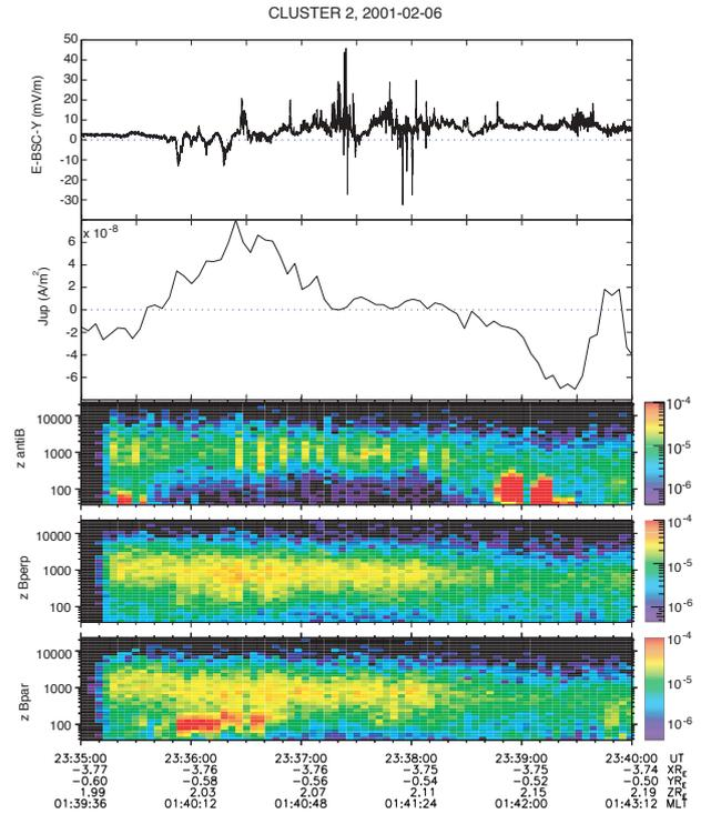
**Fig. 11.** Electron fluxes together with FACs and electric fluctuations measured by C2. From top to bottom: high-resolution electric field from the EFW, FAC (positive values correspond to current away from the ionosphere) from the FGM, and electron fluxes in the anti-parallel, perpendicular and parallel to B directions from the PEACE HEEA instrument in units of  $\text{erg cm}^{-2} \text{str}^{-1} \text{s}^{-1} \text{eV}^{-1}$  (calibration version 5).
