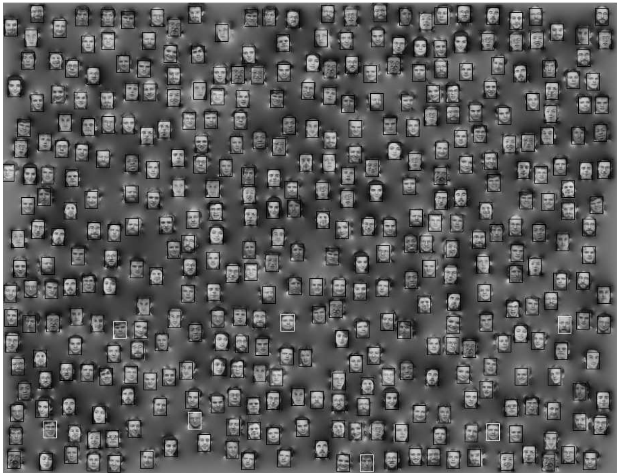
Figure 4: Propagation of the whole set of 400 initial images (belonging either to the learning base or one of the two test bases). The network is a scaled version of the one in figure 3. Here, we only presented the global result of the network superposed with the input image. A ray-tracing algorithm was used to fill the spaces between each face image in the montage. The size of the image was 910x700 pixels, which requires a network containing roughly 32 million neurons and 245 billion connections. For a correct detection, a neuron selective to a particular face must discharge within a 4x4 region located at the center of the face. Black squares indicate correct recognition and white ones false detections. Despite the size of the network, the simulation could be completed in about 30 minutes of CPU time on a modest desktop computer (Macintosh G3, 266 MHz).
