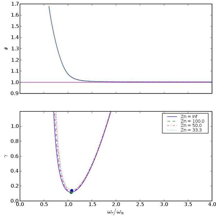
Figures 2 and 3: results for  $f_r=440\text{Hz}$  ;  $q_r=0.100$  ;  $\zeta=0.3$ , and different values of the impedance peak of the resonator. The abscissa is the ratio of the reed frequency to the resonator frequency. The upper and lower curves represent the ratio of the threshold frequency to the reed frequency, and the threshold pressure, respectively. Fig. 2(above) represents the outwards case, while Fig. 3(below) represents the inwards one.
