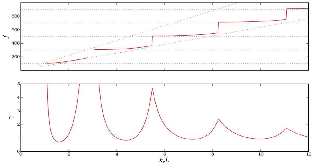
Figure 5 : results for a fixed length  $L=1m$  ;  $q_r=0.3$  ;  $\zeta=0.2$ . The abscissa is  $k_r L$ , proportional to  $\omega$ . The upper curve gives the threshold frequency, the lower curve gives the threshold pressure.
