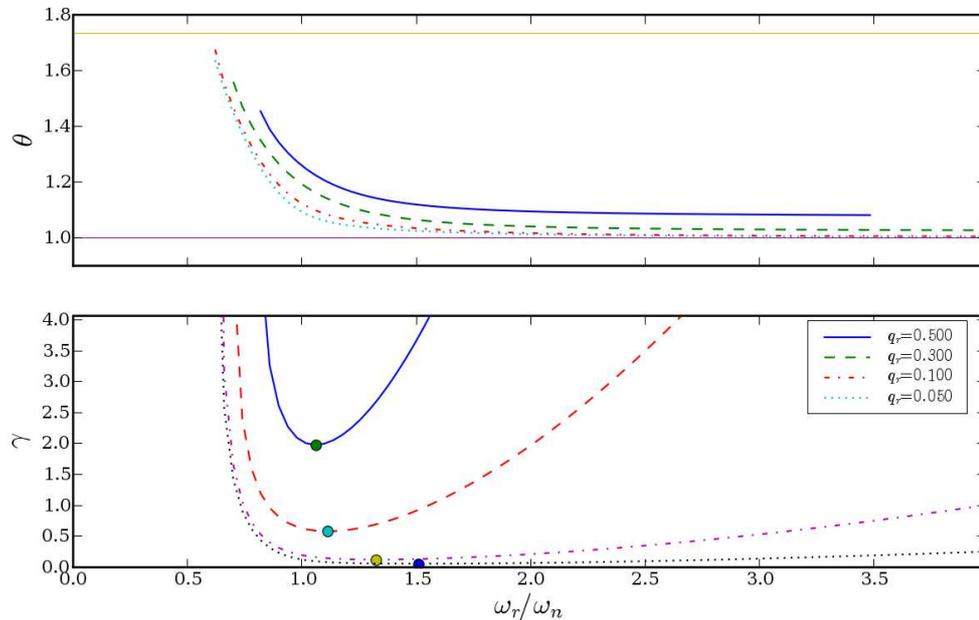
Figure 4: : results for  $f_r=440\text{Hz}$ ;  $\zeta=0.3$ ;  $Z_n=50$ , and different values of  $q_r$ . The abscissa is the ratio of the reed frequency to the resonator frequency. The upper and lower curves represent the ratio of the threshold frequency to the reed frequency, and the threshold pressure, respectively.
