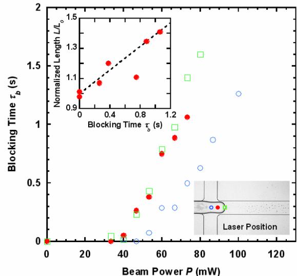
FIG. 2: (color online) Dependence of the blocking time  $\tau_b$  on laser power and position (indicated in the picture) for  $Q_{\text{water}} = 0.03 \mu\text{L}/\text{min}$  and  $Q_{\text{oil}} = 0.1 \mu\text{L}/\text{min}$ ,  $\omega_0 = 2.6 \mu\text{m}$ . Inset: Rescaled droplet length  $L/L_0$  vs. the blocking time (laser position  $\bullet$ ), where  $L_0$  is the droplet length without the laser. The dashed line is a linear fit, ignoring the outlier at  $\tau_b = 0.75 \text{ s}$ .
