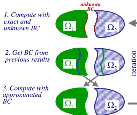
Fig.6. Basic idea of the additive Schwarz iteration.
