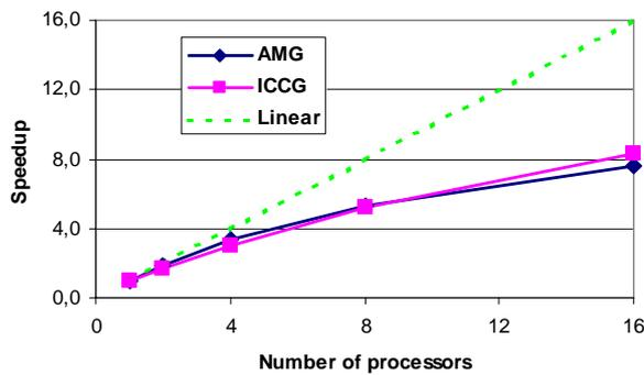
Fig. 12. Speedup of AMG and ICCG methods [19].
