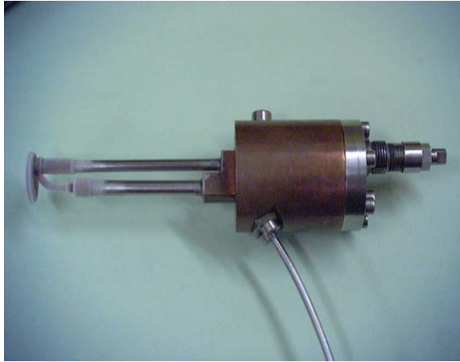
Fig. 2 Photography of the commercial DIPTR prototype (THALES CRYOGENIE) used for tests.
