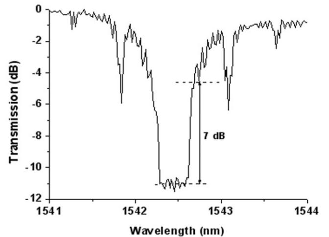
**Figure 2** Measured transmission spectrum for 5-mm-long uniform filter
