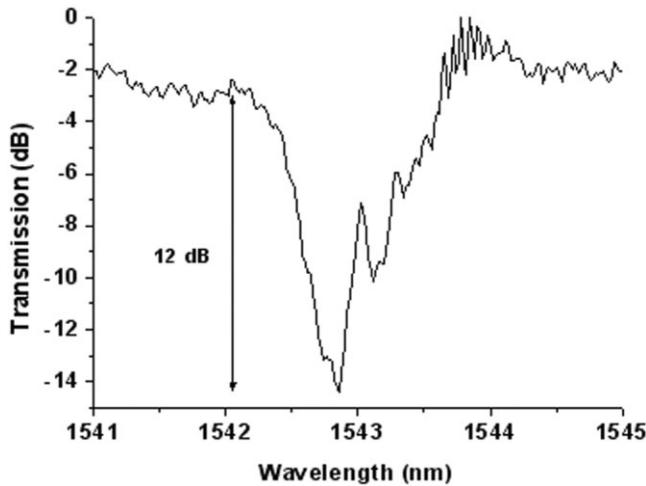
Figure 4 Transmission spectrum for the half-apodized filter
