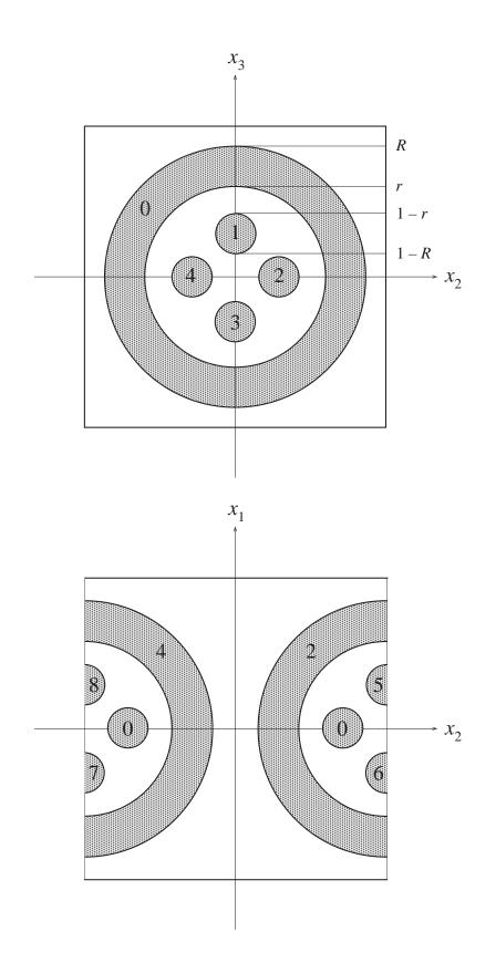
Figure 4: Sections  $x_2Ox_3$  and  $x_1Ox_2$  of the period cell: 0 is an entire link, 1, 2, 3, 4 are half-links, and 5, 6, 7, 8 are quarter-links.
