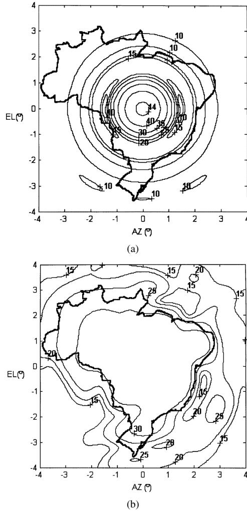
Fig. 4. Radiation pattern (in decibels): (a) reference parabolic reflector and (b) optimized shape.
