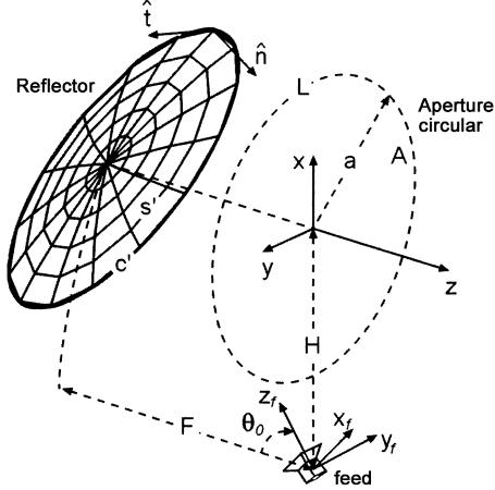
Fig. 2. Geometry of the single-feed offset reflector antenna.
