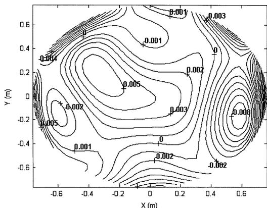
Fig.5. Difference between optimized and reference parabolic shapes.
