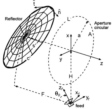
Fig. 2. Geometry of the single-feed offset reflector antenna.
