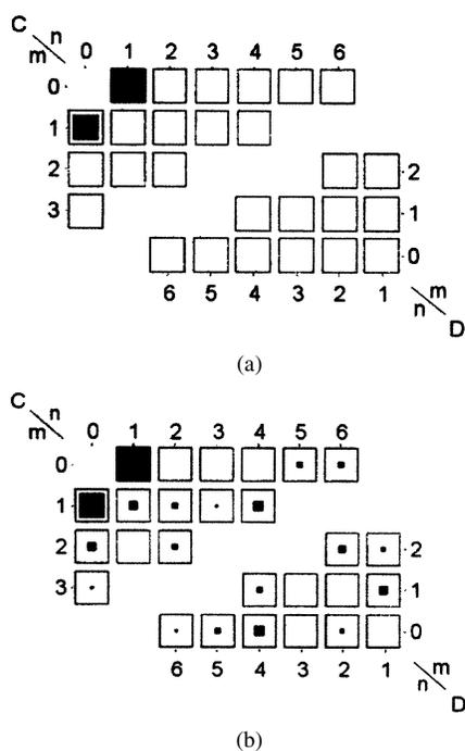
Fig. 6. Graphical representation of the 27 expansion coefficients for (a) reference paraboloid and (b) optimized shape. Diagonal of each dark square is proportional to  $\log_{10} |C_{nm}|$  (or  $\log_{10} |D_{nm}|$ ) normalized to the range  $[10^{-3}, 100]$ .
