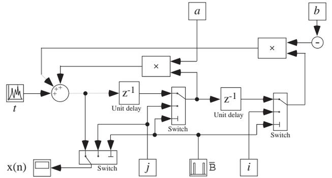
**Figure 1: A simplified second-order digital filtering system.**
