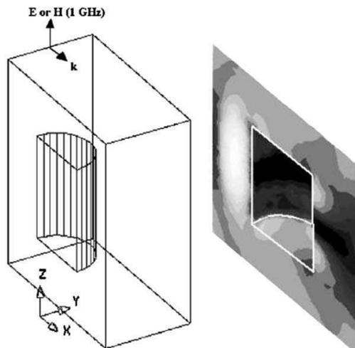
Fig. 2. Incident plane wave on a 3-D cylinder.
