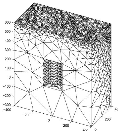
Fig. 4. Lack of uniformity for mesh 2.
