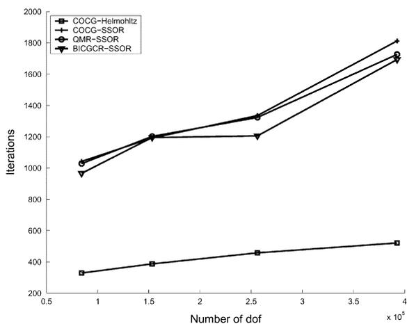
Fig. 3. Number of iterations against the number of dof.
