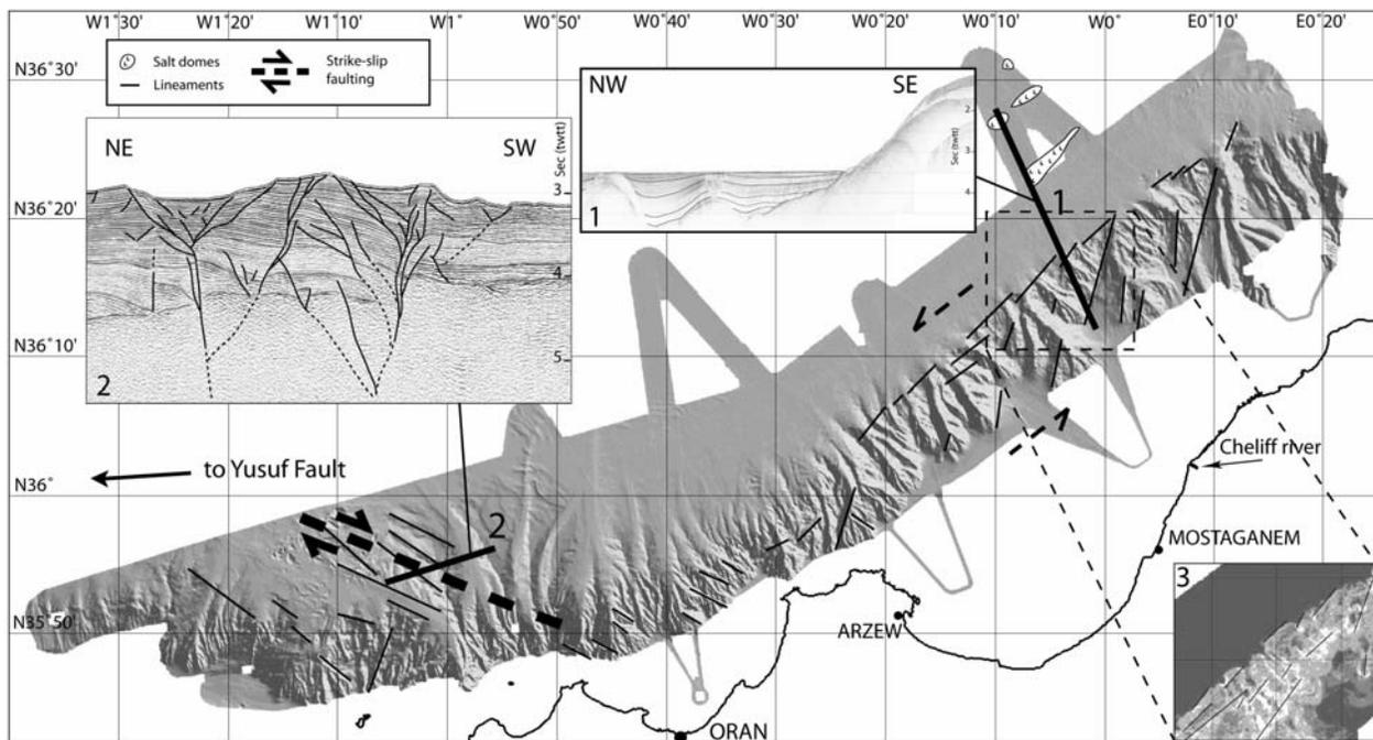
**Fig. 5.** Shaded bathymetric map (obtained from a 50-m DEM) of the Oran region with the main geological features identified (salt domes, lineaments, and strike-slip fault). Black thick lines: position of the time-migrated, stacked 6- and 24-channel seismic lines, for the seismic lines 2 and 1, respectively (vertical exaggeration: 4). Lower-right corner: slope map calculated from the 50-m DEM (slope increases from dark to white).
