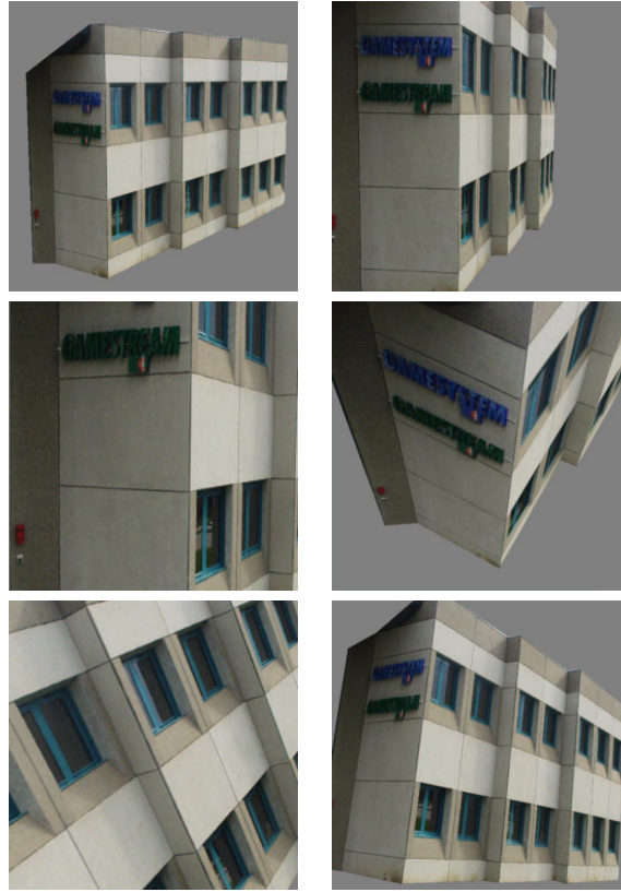
Figure 6. Textured rendering of the recovered metric model for the Game System stereo image pair.
