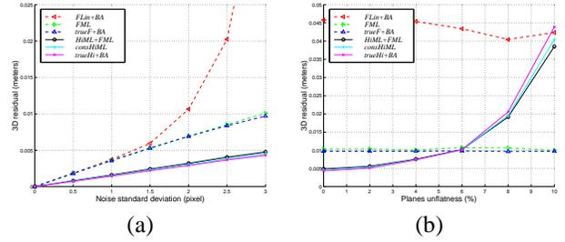
Figure 2. Comparison of the different methods using the *3D* residual  $E_3$ , for a distance scene/cameras of 10 meters and versus (a): image noise and (b): planes unflatness under a 3 pixels image noise.
