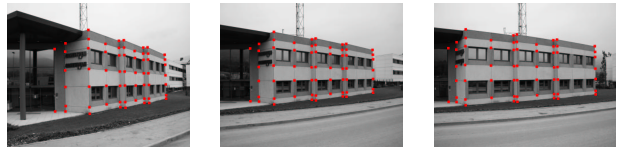
Figure 4. 3 out of the 6 actual images of an architectural scene overlaid with features. Note the significant parallax of windows relative to the wall.
